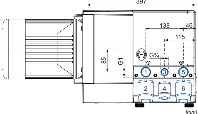
1+2 Pressure connection and pressure regulating valve
